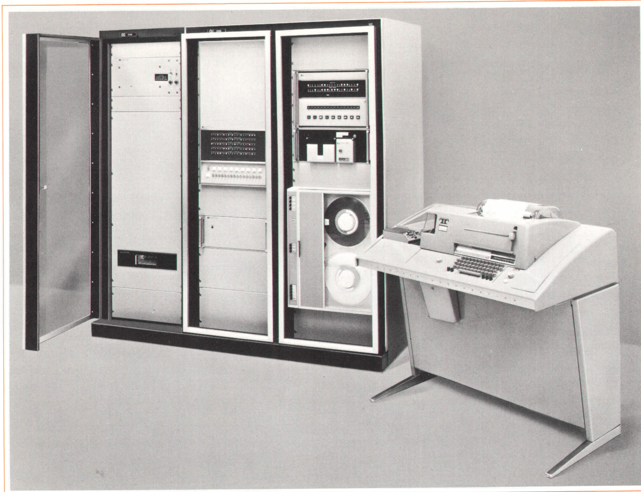
Fig. 6. The HP/CAI program runs on the HP 2000B Time-Shared Computer System. The system handles 32 students at a time. The central processor, shown here, is small enough to be located right in the elementary school, so telephone charges are minimized.
